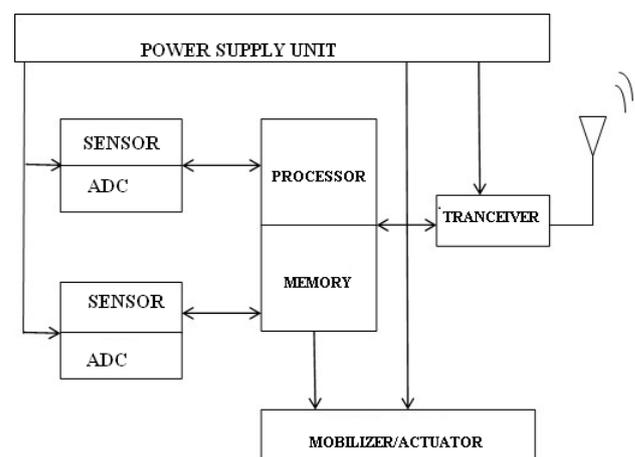
Fig.1. Typical sensor node
