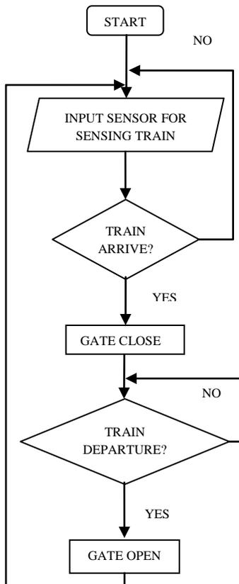
Fig. 3: Flowchart of Unmanned Level Crossing
