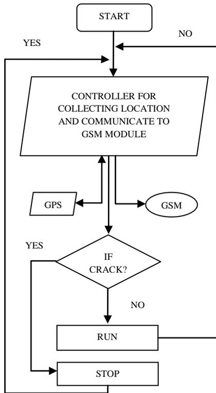
Fig 2: Flowchart of Crack Detection
