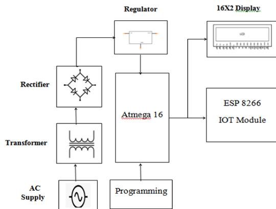
Fig. no. 1: Block diagram of the system
