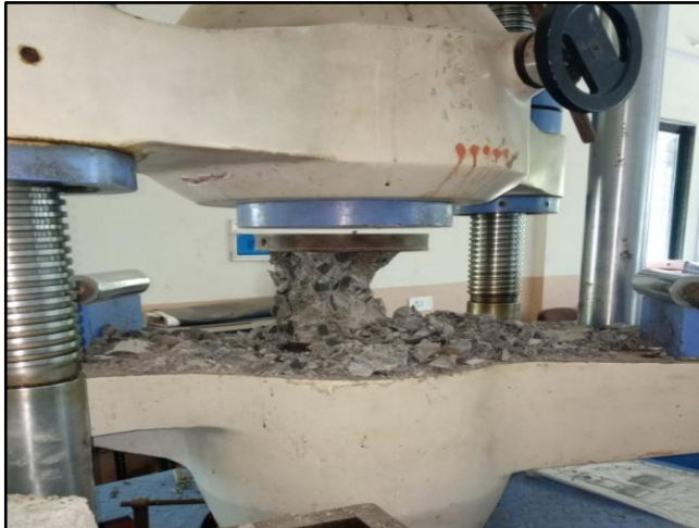
(B) Fig No. 1: (a),(b) failure of blocks after testing
