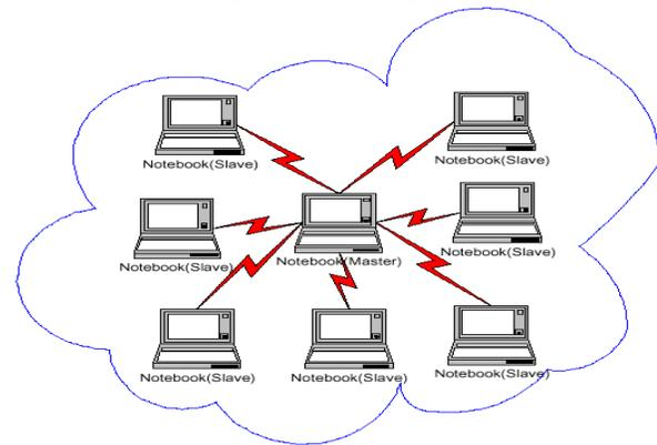
Figure 2: Single piconet ad hoc network.
