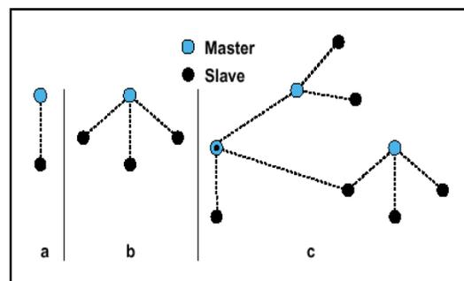
Figure 1: Piconets with single slave operation (a),
