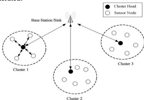
Figure 3. Cluster based sensor network.
