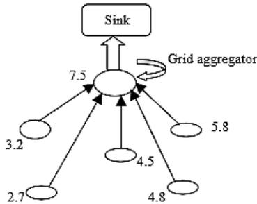
Figure 4. Grid based data aggregation scheme.
