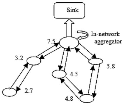
Figure 5. In-network data aggregation scheme.
