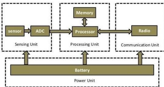
Figure 1. Architecture of sensor node
