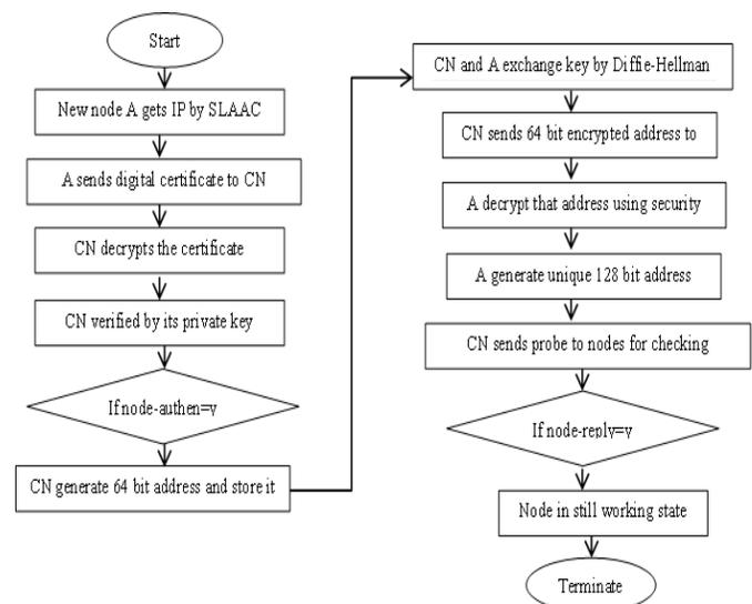
Figure 1: Flow chart of proposed method
