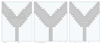
Figure 4 Geometry of UWB antenna having individual slots on radiating patch and microstrip line
