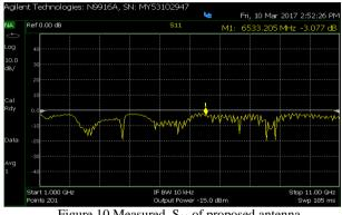
Figure 10 Measured S<sub>11</sub> of proposed antenna
