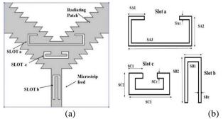
Figure 2 (a) Layout of proposed UWB antenna with three band-notched (b) Layout of the slots with its parameters Dimensions of the proposed UWB antenna with optimized parameters of antenna geometry in Fig.1 and slots shown Vol.5(2) May 2017, E-ISSN: 2321-3256
