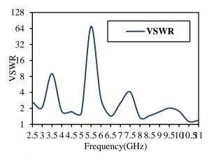
Figure 6 Simulated VSWR of proposed UWB antenna
