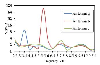
Figure 5 Simulated VSWR of UWB antennas a, b, and c.
