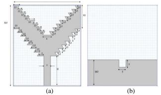
Figure 1.The design geometry of proposed initial monopole UWB antenna. (a) front view. (b)back view
