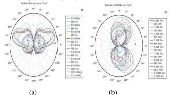
Figure 8 simulated radiation pattern in(a) E-plane (b) H- plane
