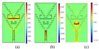
Figure 7 Simulated surface current distribution of proposed antenna at three notch frequencies (a) 3.5 (b) 5.5 and (c) 7.5GHz
