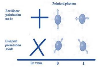
Figure 2. Polarized photons and corresponding bit values
