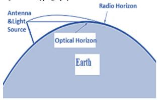
Figure 5. Optical and Radio Horizon
