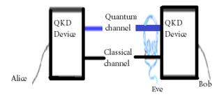
Figure1. Quantum key distribution based communication
