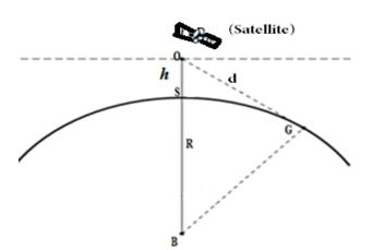
Figure-8. Quantum Key Distribution Horizon from a Satellite
