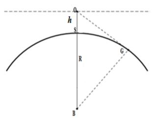
Figure-4 .Geometrical horizon calculation
